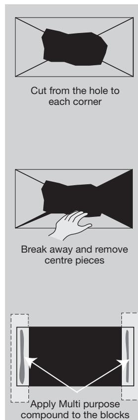
Cut 2 blocks of plasterboard that will be used as back blocks using BGC Multipurpose Joint Compound. Stick the 2 blocks of plasterboard to the inside surfaces of the wall, wiping off any excess compound. Allow 24 hours for compound to dry and harden.
